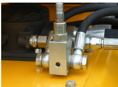
SCHOKBESTENDIGE HYDRAULISCHE BEVEILIGING SHOCK RESISTANT HYDRAULIC SAFETY DEVICE
